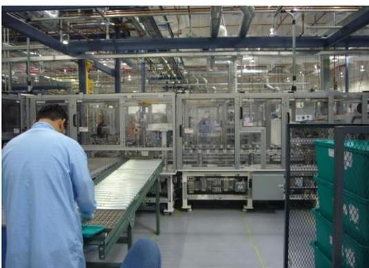
**Solyndra Kato & Page Fabs** (Fremont, CA): Factory workplace / OSHA noise control. The Owner asked us to help improve production floor noise levels. Newly-created process tools had been developed, but tool noise emissions had not yet been addressed. We measured noise levels at worker positions in the development fabs. Where problematic noise levels were encountered, we helped the Owner and tool vendors develop cost-effective mitigations for deployment in newer fabs then under construction.
