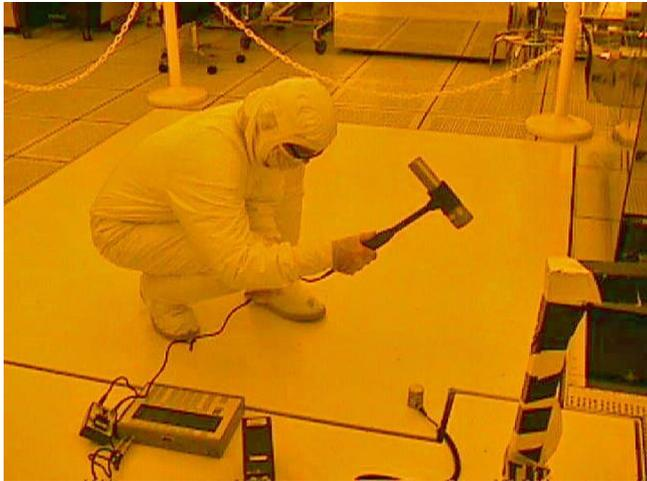
Some processes are only modestly sensitive to vibration and can be accommodated on specially-designed upper floors; however, the most demanding criteria in nanotech labs are relevant only at grade-level floors. In some cases a floating structure might be considered, but this creates significant additional expense. The existing site ambient condition, structural design, and mechanical systems all contribute to the vibration environment. In the best-case, the ambient condition limits performance.
